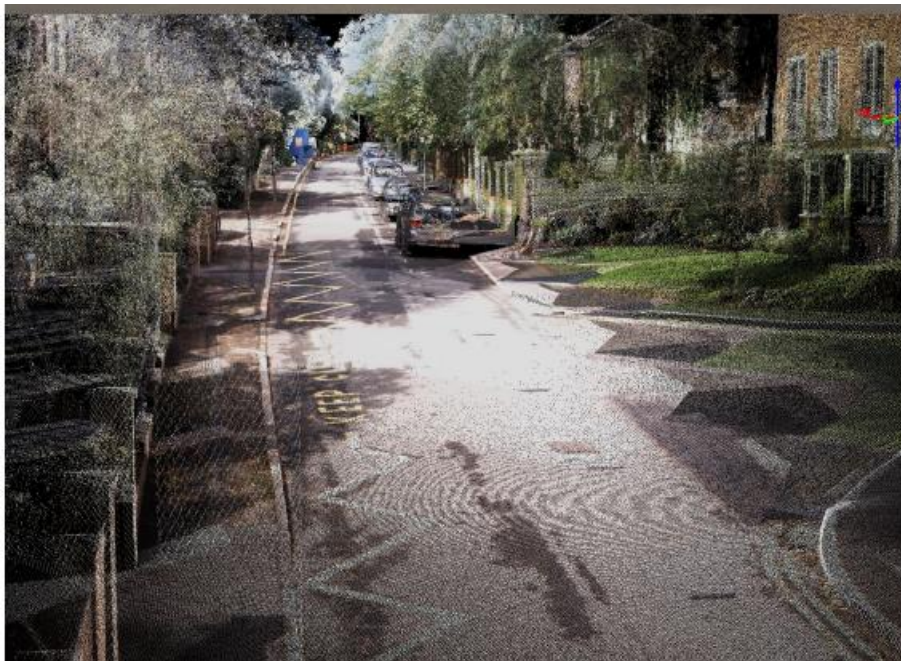
Figure 2: LIDAR laser plot plus colour camera data
