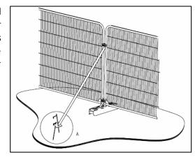
4.8 **Type 3 Tree Protection Fencing (TPF3)**, is to be erected as a visual barrier to protect areas designated for no or later construction and typically consist of light visual barriers such as stock fencing, post and rail, Chestnut Pale fencing or Orange Extruded Plastic Netting, supported on ground pins as shown opposite.
