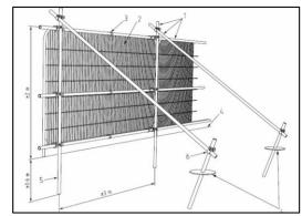
4.7 **Type 2 Tree Protection Fencing (TPF2)**, is to be erected as a temporary barrier to protect areas designated for later construction within TPZ, shall consist of Heras panels mounted on rubber/concrete 'boots' which shall be pinned into the ground using 450mm steel pins and/or clamped to adjacent Type 1 TPF, shown opposite.
