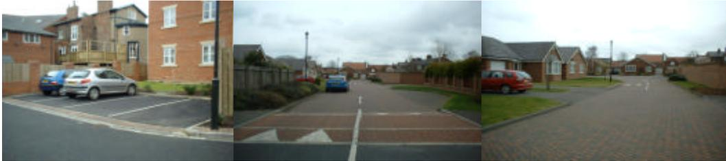
parking areas are bordered by a footway, then measures will be needed to protect it from the overhang of vehicles, or the footway widened by 800mm.
