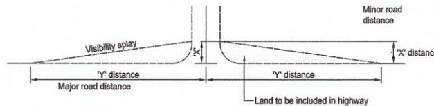
Figure 5 Visibility splays at junctions
