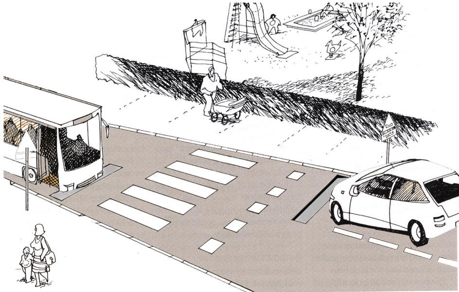
Dynamic traffic calming systems are selective. If the speed of the oncoming vehicle is above the speed limit an unevenness in the road surface is created to give the driver a physical reminder.
