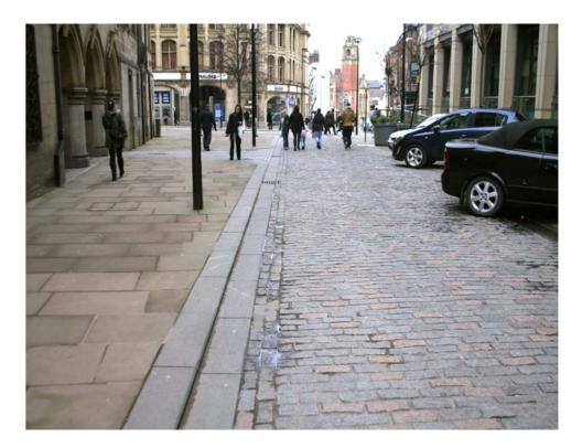
Good simple design in Sheffield using a small pallet of natural stone materials, in this case, granite setts on the carriageway, wide top granite kerbs and Marshall's Cromwell sandstone flags.
