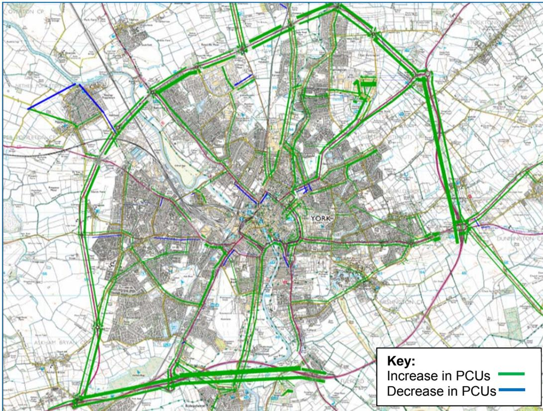
Figure 5 – PM Peak Flow Difference Plots 2010 Base and 2031 Reference Case
