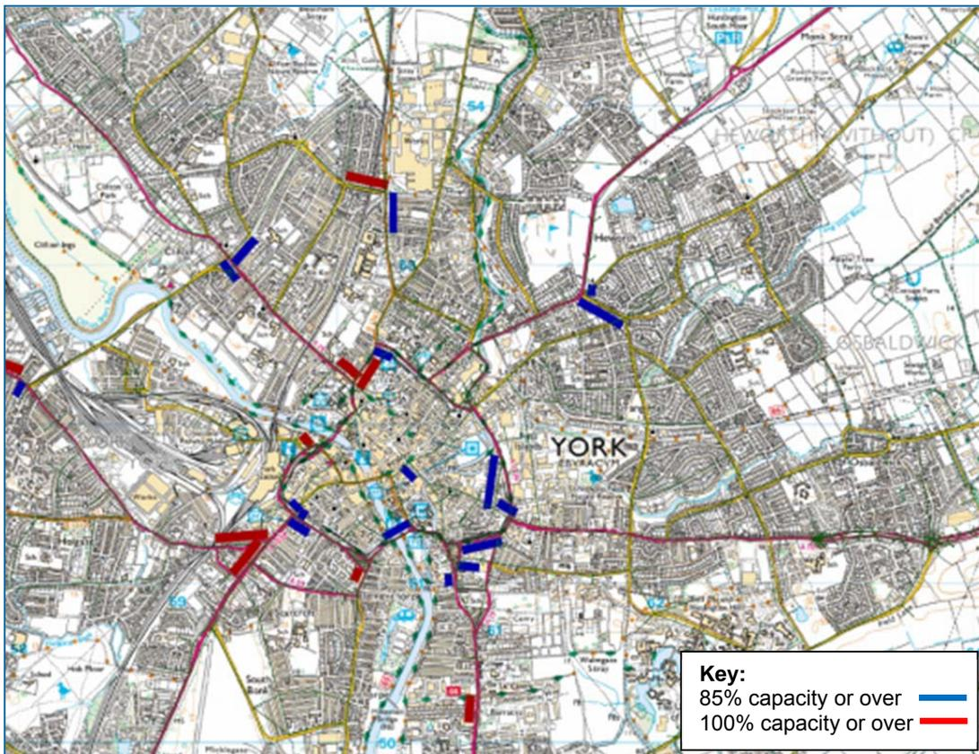
Figure 10 – 2031 AM Peak Link Capacity: Reference Case
