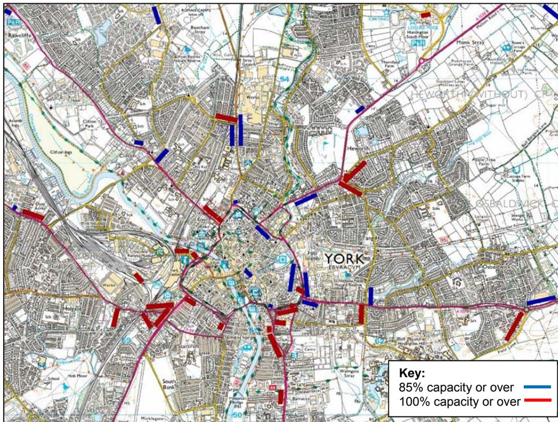
In the PM peak, the dualled A1237 greatly improves V/C on the northern section of the ORR between Wetherby Road and North Road, but anticlockwise between Strensall Road and Haxby Road still operates over capacity. This is likely due to insufficient capacity at the junctions causing vehicles to block back onto the link, reducing the effective capacity.
