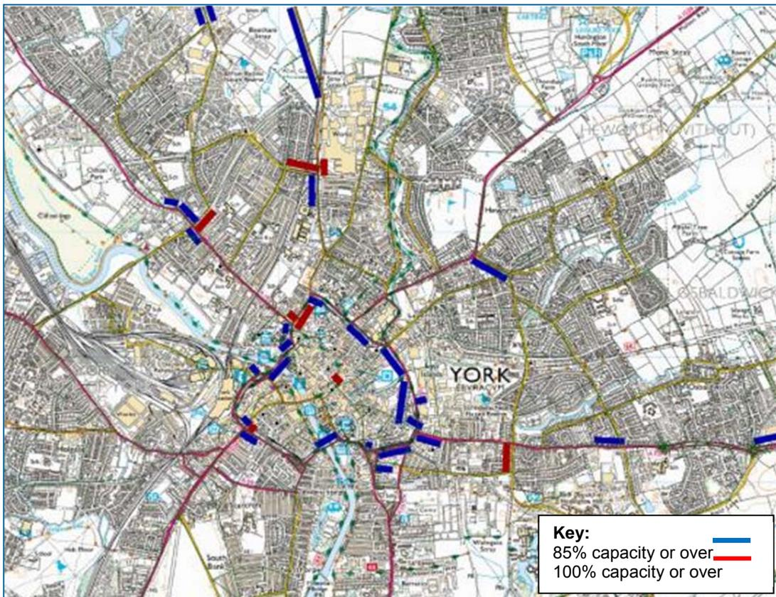
Figure 14 – 2031 PM Peak Link Capacity: Reference Case
