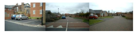
parking areas are bordered by a footway, then measures will be needed to protect it from the overhang of vehicles, or the footway widened by 800mm.
